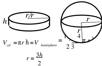
$$V_{cyl} = \pi r^2 h = V_{hemisphere} = \frac{1}{2} \cdot \frac{4}{3} \pi r^3$$
