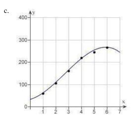
16. A V8 car engine is coupled to a dynamometer and the horsepower y is measured at different engine speeds x (in thousands of revolutions per minute). The results are shown in the table below. Use the model  $y = -1.806x^3 + 14.58x^2 + 16.4x + 30$  to approximate the horsepower when the engine is running at 5500 revolutions per minute. Round your answer to two decimal places.
