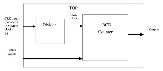
Synthesize the top module (which includes the divider and the 1-digit bcd counter) and use the following pin assignments. Download the design onto the board and make sure it works as expected.
