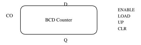
If the LOAD = ENABLE = 1, the data input D is loaded into the counter. If LOAD = 0 and ENABLE = UP = 1, the counter is incremented. If LOAD = 0, ENABLE = 1, and UP = 0, the counter is decremented. If ENABLE = 1 and UP = 1, the carry output (EO) = 1 when the counter's value is 9. If ENABLE = 1 and E = 1 and E = 1, the carry output (E = 1) when the counter's value is 0.
