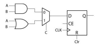
Unlike Clr, the output from the mux is only read on falling clock edges; therefore, adding C to the sensitivity list is not required for proper operation of the circuit.
