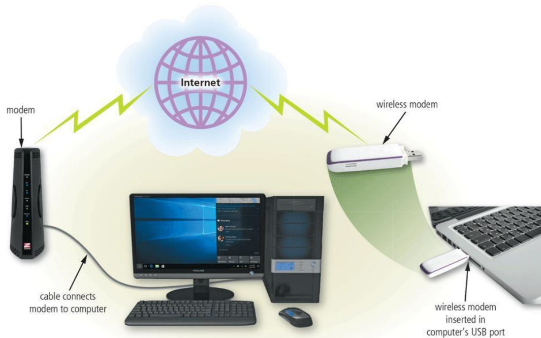
Figure 2-2 Using a modem is one way to connect computers and mobile devices to the Internet. Courtesy of Zoom Telephonics Inc; Oleksiy Mark / Shutterstock.com; Source: Microsoft; Kristina Postnikova / Shutterstock.com; Kristina Postnikova / Shutterstock.com; DR / Fotolia LLC
