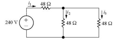
Write a KVL equation for the left and right loops:
