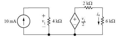
$$v_1 = (4000)(0.01) = 40 \text{ V}$$
