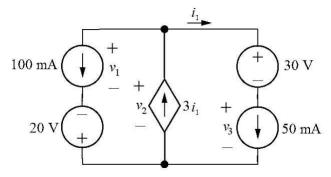
The voltage drop across the left branch, the center branch, and the right branch must be the same, since these branches are connected at the same two terminals. This requires that
