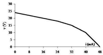
**[b]** Since the plot is linear for  $0 \le i_S \le 24$  mA amd since R = v/i, we can calculate R from the plotted values as follows:
