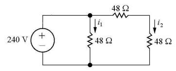
Write a KVL equation for the left and right loops:
