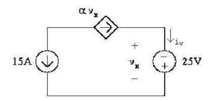
[a] Note from the circuit that  $v_X = -25$  V. To find  $\alpha$  note that the two current sources are in the same branch of the circuit but their currents flow in opposite directions. Therefore
