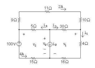
$$v_2 = 100 + 4(15) = 160 \text{ V};$$
