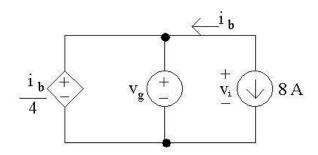
[a] Note that the current i<sub>b</sub> is in the same circuit branch as the 8 A current source; however, i<sub>b</sub> is defined in the opposite direction of the current source. Therefore,
