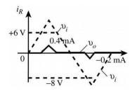
37. (a) Starting with  $v_i = 20 \text{ V}$ , the diode is in the "on" state and the capacitor quickly charges to 20 V+. During this interval of time  $v_o$  is across the "on" diode (short-current equivalent) and  $v_o = 0 \text{ V}$ .
