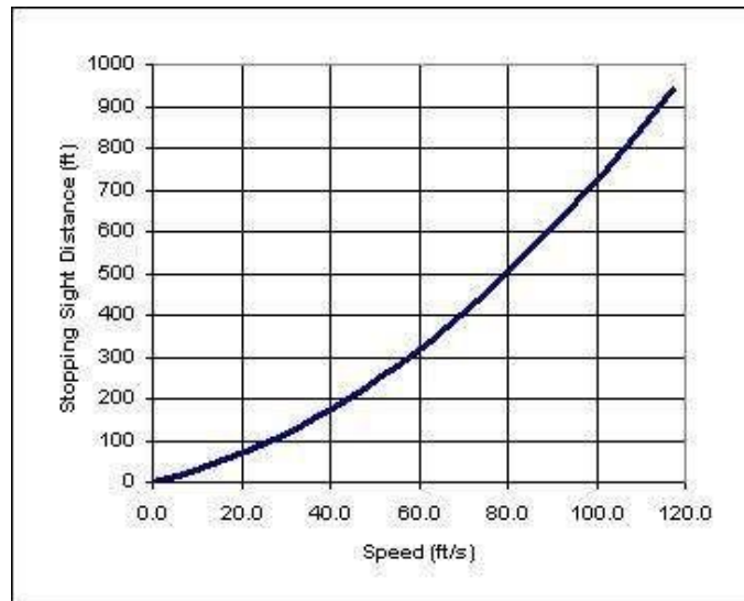
Figure 4.17 The stopping sight distance for a car traveling up to speed of 80 mph.
