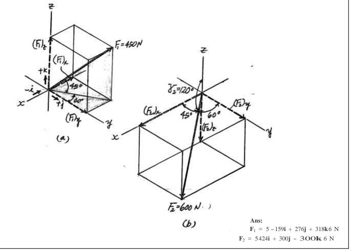
**2–61.** Determine the magnitude and coordinate direction angles of the resultant force acting on the bracket.
