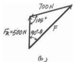
F = 960 Nu = 45.2 **2–6.** If  $F_B = 2 \text{ kN}$  and the resultant force acts along the positive *u* axis, determine the magnitude of the resultant force and the angle u.
