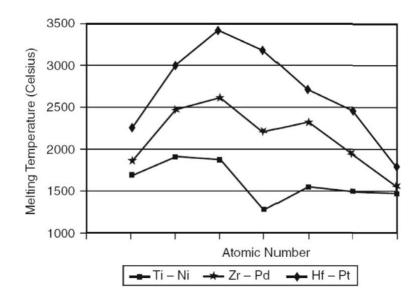
For each row, the me lting temperature is hig hest when the outer "d" energy lev el is partly full. In Cr, t here are 5 electrons in the 3d shell; in Mo, there are 5 electrons in the 4d shell; in W there are 4 electrons in the 5d she ll. In each c olumn, the melting tem perature in creases as the atomic number increases—the at om cores contain a larger number of tightly held electrons, making the metals more stable.
