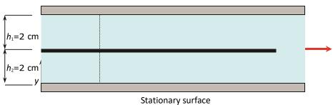
The magnitudes of shear forces acting on the upper and lower surfaces of the moving thin plate are
