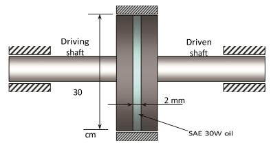
Analysis The disks are rotting in the same direction at different angular speeds of  $\omega_1$  and of  $\omega_2$ . Therefore, we can assume one of the disks to be stationary and the other to be rotating at an angular speed of  $\omega_1 = \omega_2$ . The velocity gradient anywhere in the oil of film thickness h is V/h where  $V = (\omega_1 - \omega_2)r$  is the tangential velocity. Then the wall shear
