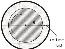
Assumptions 1 The inner cylinder is completely submerged in oil. 2 The viscous effects on the two ends of the inner cylinder are negligible. 3 The fluid is Newtonian.
