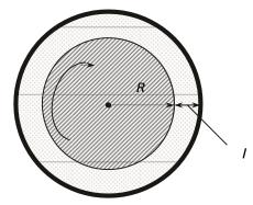
Analysis (a) The radius of the shaft is R = 0.05 m, and thickness of the oil layer is  $\Box = (10.3 - 10)/2 = 0.15$  cm. The powertorque relationship is
