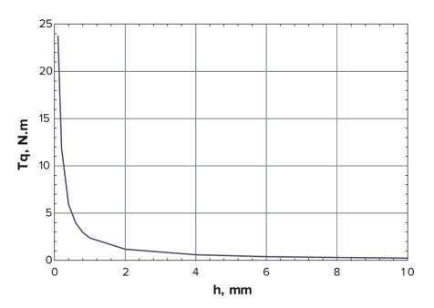
**Conclusion** Torque transmitted is inversely proportional to oil film thickness, and the film thickness should be as small as possible to maximize the transmitted torque.
