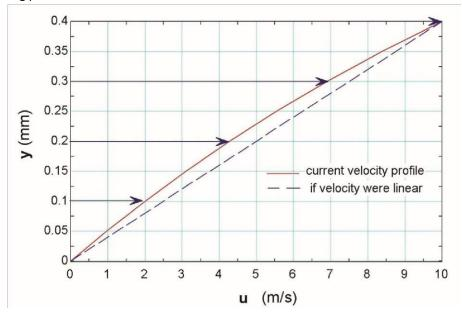
(b) Using Newton's law of viscosity
