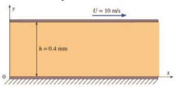
Analysis (a) Taking an infinitesimal fluid element and applying force balance (assuming one dimensional flow),
