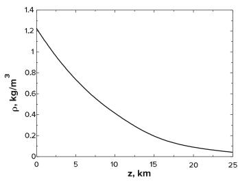
Analysis Using EES, (1) Define a trivial function "rho= a+z" in the Equation window, (2) select new parametric table from Tables, and type the data in a two-column table, (3) select Plot and plot the data, and (4) select Plot and click on curve fit to get curve fit window. Then specify  $2^{-n}$  order polynomial and enter/edit equation. The results are:
