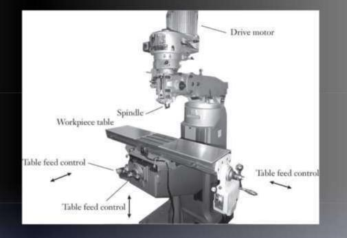
The workpiece is held by a vise on an adjustable table so that the part can be accurately moved in three directions.
