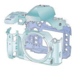
This was most likely manufactured using a die cast procedure because of the material and geometric detail in the pieces including a number of inclusions. Certain features could have been machined, and some polishing/grinding operations may have been used.
