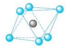
The combination of the octahedral aluminum hydroxyl units give an octahedral sheet.
