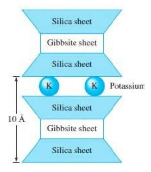
Montmorillonite has a similar structure to illite—that is, one gibbsite sheet sandwiched between two silica sheets.
