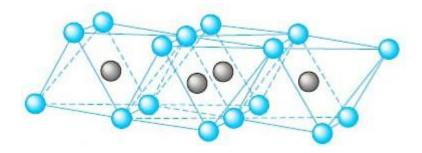
Kaolinite consists of repeating layers of elemental silicagibbsite sheets, as shown in the figure below.
