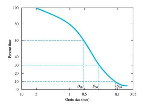
Three basic soil parameters can be determined from these curves, and they can be used to classify granular soils.
