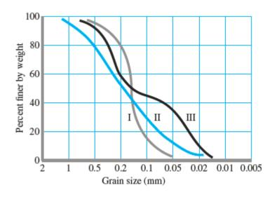
Curve I represents a type of soil in which most of the soil gains are the same size. This is called poorly graded soil.
