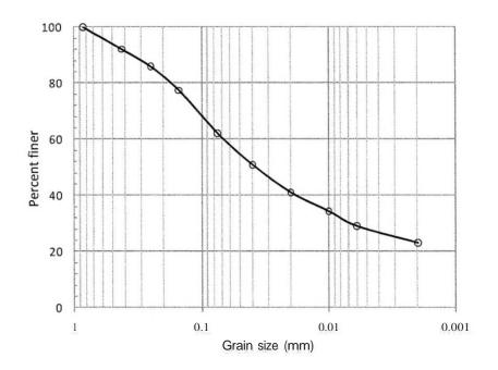
From the figure: Percent finer than 2 mm = 100% Percent finer than 0.06 mm= 58% Percent finer than 0.002 mm= 23%
