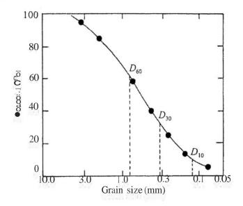
b. From the figure , Dao = 0.82 mm, D3% = 0.31 mm, Do = 0.12 mm
