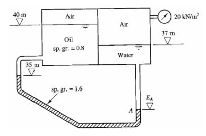
Ans. Using the "swim through" technique, start at the right tank where pressure is known and "swim through" the tanks and pipes, adding pressure when "swimming" down and subtracting when "swimming" up until you reach the known pressure in the left tank. Solve for the variable elevation ( $E_A$ ) in the resulting equation.
