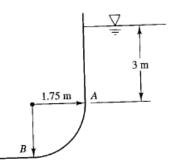
Ans.  $F_H \cdot \cdot \cdot \overline{h} \cdot A = (1.03)(9790 \text{ N/m}^3)(3.875 \text{ m})[(1.75 \text{ m})(1\text{m})] = 68.4 \text{ kN}$  (per unit length of hull)
