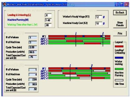
5. A study revealed that a group of three semiautomatic machines assigned to one operator operate 70 percent of the time unattended. Operator service time at irregular intervals averaged 30 percent of the time on these three machines. What would be the estimated machine hours lost per eight-hour day because of lack of an operator?
