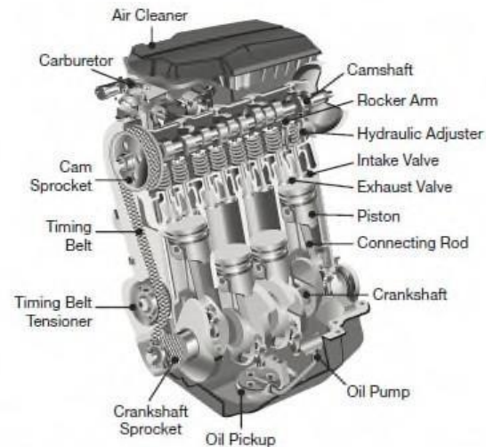
FIGURE 2.22 Rotating shaft work can be found in many devices, including a turbine and the crankshaft of a reciprocating engine.
