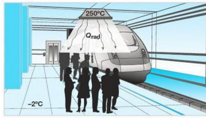
FIGURE 2.15 Heat lamps use radiative heat transfer to keep people warm in outdoor
