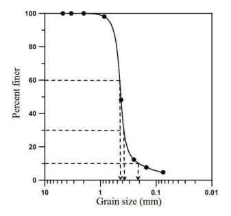
b.  $D_{10} = 0.21 \text{ mm}; D_{30} = 0.39 \text{ mm}; D_{60} = 0.45 \text{ mm}$
