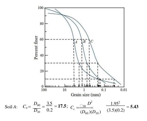
Although  $C_u > 6$ ,  $C_c$  is not between 1 and 3. The sand is **poorly graded**.
