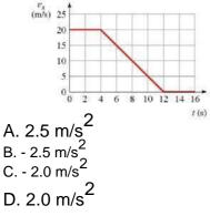
29. The figure shows the graph of v<sub>x</sub> versus time for an object moving along the x-axis. What is the acceleration at t = 7.0 s?
